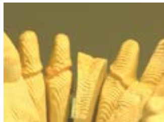
Fig. 19 Strip light projection of the laboratory scanner Lava Scan ST (3M Espe)
