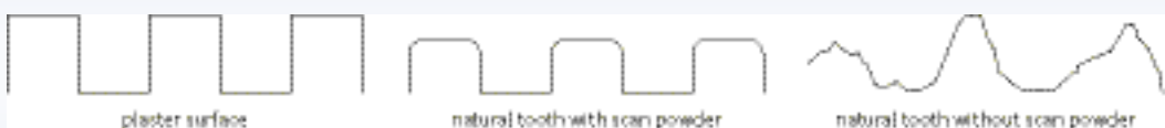
Fig. 15 Brightness distribution in the differential image with strip light projection. The quality of the signal of the strip light projection depends strongly on the surface condition (for example, reflection of a glossy surface).
