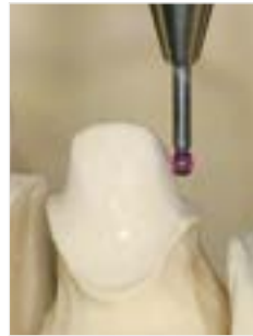
Fig. 26 Probe of the Nobel Procera Forte (Photo: Nobel Biocare)
