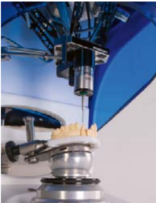
Fig. 2a & b Principle of a tactile measuring probe system (Photos: Renishaw)
